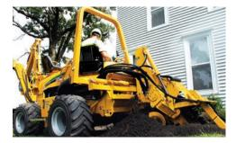
TIRE OPTIONS. The RTX550 is available with standard 31" (78.7 cm) tires. For even greater flotation, choose the 35" (88.9 cm) tire option. Additionally, the ride-on tractor is available with quad tracks which are ideal for uneven terrain.
