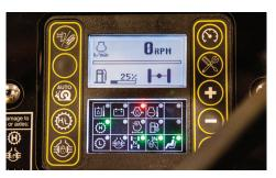
**KNOWLEDGE ON DISPLAY.** An integrated system display toggles through machine diagnostics, including engine rpm, fuel level, alternator voltage, engine coolant temperature and engine hours. When in either ground drive or using a rear attachment, the display indicates the percentage of the hydrostatic capacity being utilized, allowing the operator to easily monitor important machine functions.
