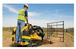
A DEDICATED SPRING-CUSHIONED **PLATFORM** keeps the operator out of the mud. The integrated operator presence system suspends ground drive and powered boom/bucket motion when the operator steps off the platform.
