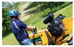
**TWO-SPEED GROUND DRIVE.** The operator may choose a high-range or low-range ground speed setting of 0 - 133 fpm (0 - 40.5 m/min) to quickly move the machine or choose a slower speed when near the stump by utilizing a low-range setting of 0 - 66 fpm (0 - 20.1 m/min).
