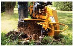
AUTOSWEEP® CONTROL SYSTEM. When equipped, the AutoSweep system monitors engine speed and automatically adjusts cutter wheel sweep rate, and is designed to reduce engine, drivetrain and structural stress.
