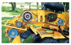
**CONVENIENT BELT SERVICING.** Belts on the SC292 are serviceable from one side of the machine with cutter drive belts being adjustable with movable idlers. Additionally, each belt set may be adjusted independently without affecting adjustment of other belts.
