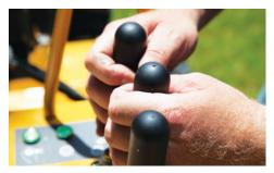
**OPERATOR PRESENCE SYSTEM.** Control handles for the boom swing, boom raise/lower and machine propel are equipped with an operator presence handle design which provides capacitance-sensing capability. This user-friendly operator presence system is intended to help protect the operator and enhance operator safety.
