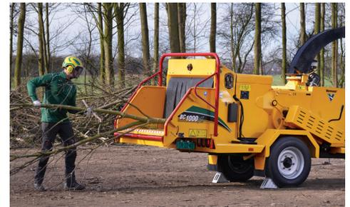
**PATENTED SMARTFEED SYSTEM.** The patented SmartFeed system helps to increase operator productivity while reducing strain on vital engine parts. The feed-sensing control system monitors engine rpm and automatically stops and reverses the rollers when feeding larger, hardwood material.
