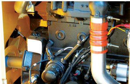
**POWERFUL PERFORMANCE.** The Cummins B3.3 turbo Stage IIIB engine delivers 55 kW (74 hp) of power for excellent performance.
