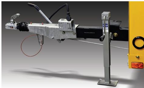
**EUROPEAN HITCH AND SURGE BRAKE.** The full type approved European undercarriage comes with a Knott axle and surge brake. The heavy-duty undercarriage provides good towing performance on-road.
