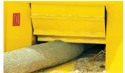
**FEED ROLLER.** A large letterbox infeed opening (44 cm x 30 cm) helps boost productivity by reducing the need to trim material before feeding it into the chipper.
