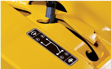
**CLUTCHLESS PTO SYSTEM.** A clutchless PTO system allows the cutter to be engaged without using a traditional slip clutch or idler pulley and without sliding the engine. The system is simple to maintain - once under the shield, belt changes are easily accomplished without the use of tools.
