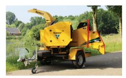
CONVENIENT 180° SLEW RING. Allows the chipper infeed to be rotated to face the material for ease of feeding and convenience when working along the roadside.
