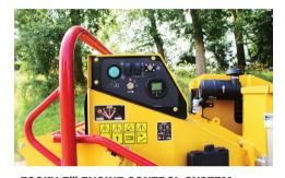
**ECOIDLE™ ENGINE CONTROL SYSTEM.** When the Ecoldle system is selected by the operator, the engine speed automatically lowers to a preset rpm after 1 minute or 5 minutes of inactivity to help reduce fuel consumption when not chipping material. This idling can help reduce emissions and noise.
