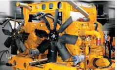
**ONE CAT IS NOT ENOUGH.** The T1655III features two CAT C18 ACERT engines providing 1200 hp (895 kW) to muscle through the toughest conditions.
