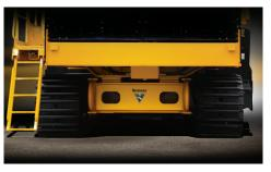
**MOBILITY AND STABILITY.** The T1655III dual tracks and low center of gravity allow for maneuverability and stability over the changing and diverse surface conditions.
