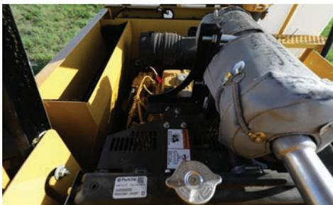
**POWERFUL PERFORMANCE.** The MX300D is equipped with a 24.7-hp (18.42-kW) CAT C1.1 engine and 350-gpm (1,324.9-L/min) pump flow to provide powerful performance on the job.
