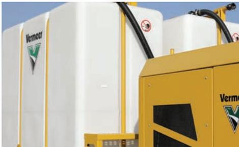
**CONVENIENT CONFIGURATION.** The MX300D comes with two tanks, powered by the same power unit, to provide more fluid onsite, with the option to support either the 750-gal (2,839.1-L) or the 1,000-gal (3,785.4-L) tank. The tanks can run independently, or together, depending on fluid amount needed.
