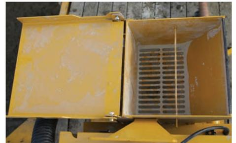
**A CLEAN MIX.** A wide-mouth hopper pairs with the tapered bottom rectangular tank to help prevent drilling fluid additives from settling, assist with drainage and reduce buildup.
