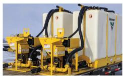
**CONVENIENT CONFIGURATION.** Configure the setup to fit your jobsite needs - arrange two units on one trailer or even pair up to two tanks with one power unit to provide more fluid onsite with the option of the TK750 tank with 750 gal (2,839.1 L) or the TK1000 tank with 1000 gal (3,785.4 L).
