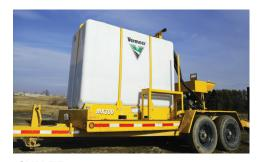
SLIM FIT. The MX300 has a tank design that is 105" (266.7 cm) long and 40" (101.6 cm) wide. This slim rectangular profile allows for convenient transport of up to two tanks inside an enclosed truck.
