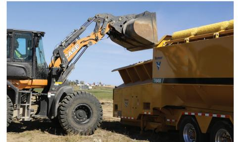
**LOW HOPPER HEIGHT.** With a hopper height of 9.5 ft (2.9 m), the operator can load material without having to build a ramp to the machine, decreasing loading cycle times.
