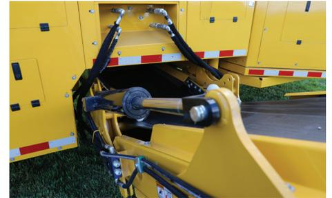
**JOB SITE FLEXIBILITY.** The auxiliary hydraulic system grants the TR6450 trommel screen the ability to run the third fraction conveyor or other attachments.
