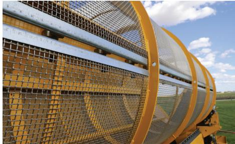
**TENSIONED SCREEN DRUM.** Tensioning the screens allows for maximum strength with a fine wire gauge, optimizing production through improved open area. In high moisture applications, the use of stainless steel screens can be very useful.
