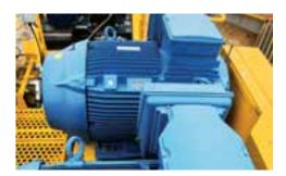
**ELECTRIC MOTORS.** The HG6000E is powered by two electric motors that deliver a combined 700 hp (522 kW) to the mill. A separate 60 hp (45 kW) electric motor powers the pump for the hydraulic circuits, while a 2 hp (1 kW) electric motor is used to cool the hydraulic system.
