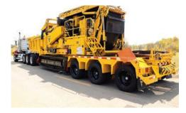
**MOBILITY.** The track-driven grinder offers onsite mobility, with a remote control for easy maneuverability. The DT6 optional integrated dolly transport system eliminates the need for a dedicated trailer to move between sites.
