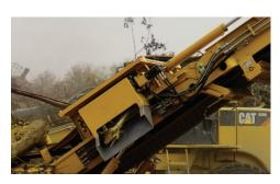
**OVERBAND MAGNET.** An optional, overband helps remove ferrous material from the end product.
