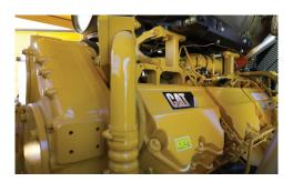
ENGINE POWER. A CAT C32 Tier 4 Final Stage V engine provides 1,125 hp (839 kW) of power to meet your jobsite demands.
