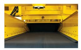
**HIGH PRODUCTION.** Smooth, 63-in (160-cm) belt enables high-volume product removal and is constructed of .5-in (1.3-cm) thick rubber belt to help resist tearing and puncturing.
