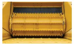
**POWERFUL FEED ROLLER.** The feed roller is equipped with aggressive teeth, coupled with down pressure, that provide pull in power and maintain control of the material being fed to help get the job done efficiently. The feed roller drive planetary is fully enclosed for protection from debris and also allows for a tight clearance between the feed roller and mill housing. This helps minimize material blockage and reduces the power required to feed material.
