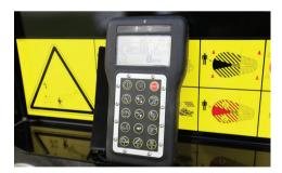
**COMPLETE CONTROL.** A state-of-the-art wireless remote control unit allows the operator to run most machine functions from up to 300 ft (91.4 m) away. This lets the operator, from the cab, adjust machine settings as the materials change, including control of the infeed settings, engine droop, conveyor height and more. Operators can spend more time in the cab throughout the day, and make machine adjustments quickly.
