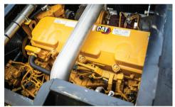
**CAT ENGINE POWER.** The 536 hp CAT C13B engine provides the horsepower needed for processing difficult materials, while also enabling worldwide service and support for maximum productivity.
